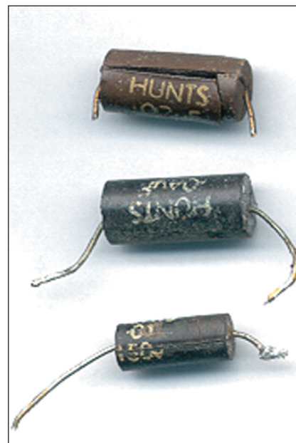
Hunts plastic capacitors – many restorers replace these on sight.
