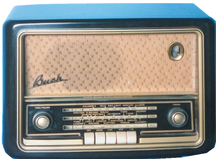
Bush VHF61 AM/VHF set from 1956 sporting a magic-eye tuning indicator.
