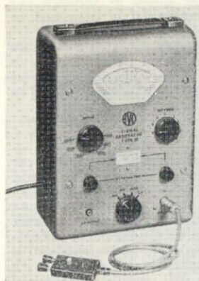
FIG. 5—AVO SIGNAL GENERATOR. This A.M./C.W. signal generator covers 150 kc/s to 220 Mc/s in six ranges.
