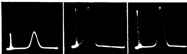
Figs. 43, left, 44, middle, and 45. When aligning at 600 kc., the peak should have maximum amplitude, regardless of its position on the trace. The oscillogram of Fig. 43 is incorrect, as the amplitude is too small when compared with that of Fig. 44, even though the curve is off center. The curve was centered, Fig. 45, by changing the receiver tuning from 600 kc. to 595 kc.
