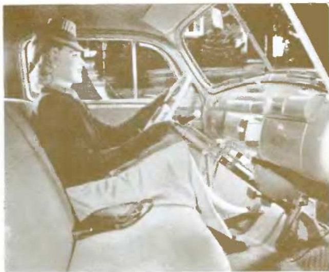
Foot switch for changing stations was a Zenith car radio tuning advance. It followed earlier innovations like the steering column tuning control.
