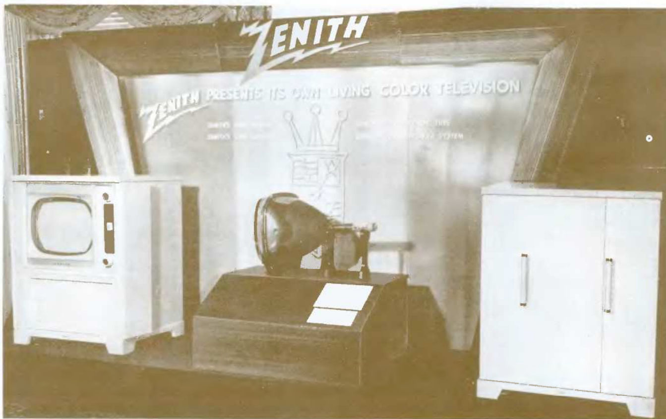
Color TV research and development by Zenith and Rauland provided the first 21-inch rectangular 3-gun color tube in 1954.
