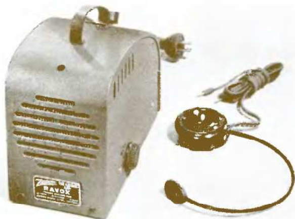
Designed for home and office use, the Ravox hearing aid operated on house current.
